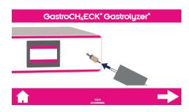
The device will then illustrate to attach the breath bag. Ensure to carefully remove the blue plug on one end only and attach the bag to the moisture filter, then open the clamp on that end only to preserve the sample.
