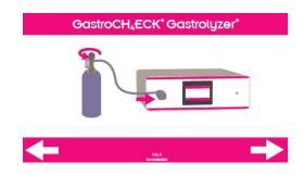
Attach the CaliAdaptor to monitor via the sample line and open the gas canister. Press the arrow to begin the calibration.
