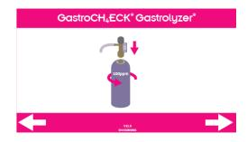
Screw the gas canister into the regulator.
