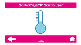
The temperature of the GastroCH<sub>4</sub>ECK® is below 17°C and is too cold to be calibrated. Please move the device to a warmer area and try again later.
