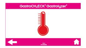
The temperature of the GastroCH<sub>4</sub>ECK® is above 25°C (77°F) and is too hot to be calibrated. Please move the device to a cooler area and try again later.
