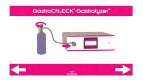
Attach the CaliAdaptor to monitor via the sample line and open the gas canister. Press the arrow to begin the calibration.
