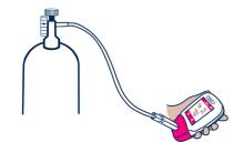
As prompted, attach the regulator to the Gastro<sup>+™</sup> device and follow the onscreen instructions to run the calibration
