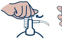
Close the regulator when the calibration is finished
