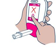
If the the Gastro<sup>+™</sup> Gastrolyzer® failed its calibration a red cross will show, press the retry icon to try again. If unsuccessful consult the troubleshooting section of the manual or contact your local distributor for help
