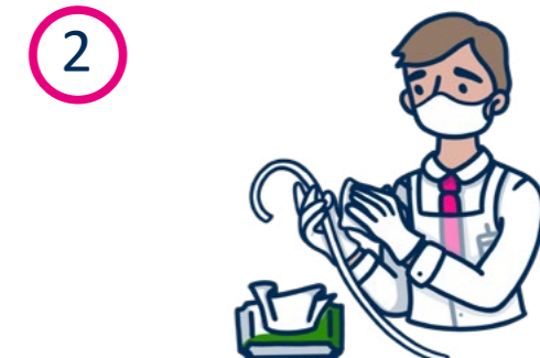
The external surfaces of the sample line should also be wiped down before and after each test
