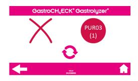
CH<sub>4</sub> sensor connectivity error: Press the retry button. If the error occurs more than 3 times, please restart the device. If failure persists contact Bedfont® or their distributor for support.
