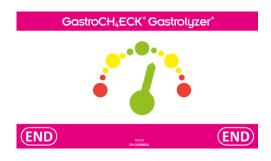
The arrow will change colour as the  $O_2$  level in the breath sample reduces to the target 15%, at which point it will turn green and the test will automatically stop after 3 seconds.
