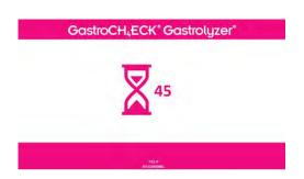
Once zeroed, breath bag sampling will begin automatically – make sure that the clamp is open. At this point, the device needs no further intervention until a reading is recorded.
