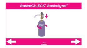
Screw the gas canister into the regulator.
