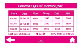
**NOTE:** Calibration errors will only appear in the log and not as a separate warning. The possible errors are:
