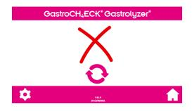
Calibration failed: Check calibration gas tubing is connected to the breath sampling port.
