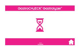
A timer will be shown onscreen whilst the sensors are zeroing. This may take up to 75 seconds if a test has just been carried out.
