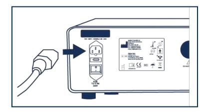
3. Switch the device on using the ON/OFF switch at the back of the device. The screen will light up and if any warning screens are displayed, these should be checked in the Troubleshooting section of the manual.
