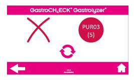
CH<sub>4</sub> sensor reading error: Verify that no gas is flowing through the device. If gas was being used, please wait 5 minutes before attempting a new test and then press the retry button. If the error occurs more than 3 times, please restart the device. If failure persists contact Bedfont® or their distributor for support.
