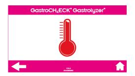
The temperature of the GastroCH<sub>4</sub>ECK® is above 25°C (77°F) and is too hot to be calibrated. Please move the device to a cooler area and try again later.
