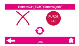
CH<sub>4</sub> sensor failure: Press the retry button. If the error occurs more than 3 times, please restart the device. If failure persists contact Bedfont® or their distributor for support.
