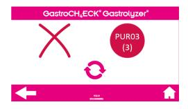
CH<sub>4</sub> sensor error: Check that the ambient temperature is within range and that the device is plugged correctly. Then press the retry button. If the error occurs more than 3 times, please restart the device. If failure persists contact Bedfont® or their distributor for support.
