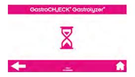
A timer will be shown onscreen, whilst the sensors are zeroing. This may take up to 75 seconds if a test has just been carried out.
