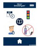
Press the calibration icon 5 times to enable.
