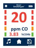
If a high reading has been recorded, the device can be muted by the sound by pressing the volume icon.
