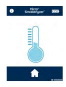
If the temperature of the device is too low to calibrate, the blue thermometer will be shown. Try again later once the unit has warmed up – if this problem persists, please contact Bedfont® or the local supplier.
