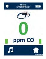
The Micro<sup>+™</sup> will then carry out real-time monitoring of the environmental air. To stop the test, press the home icon.
