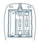
Ensure that the batteries are inserted the correct way around, matching the symbols moulded into the plastic.
