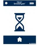
The device may show this screen when the sensor is zeroing.
