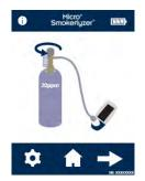
Insert a D-piece™ into the device and turn on the gas. Press the arrow to continue.
