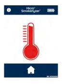
If the temperature of the device is too high to calibrate, the red thermometer will be shown. Try again later once the unit has cooled down – if this problem persists, please contact Bedfont® or the local supplier.
