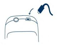
Place one end of the connection lead into the USB socket on the top of the Smokerlyzer® product.
