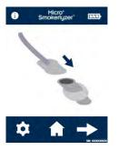
Attach a D-piece™ to the calibration adaptor. Press the arrow to continue the calibration process.
