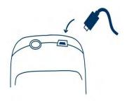
Place one end of the connection lead into the USB socket on the top of the Gastro+™ Gastrolyzer® product.
